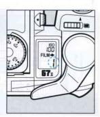
4. Depress the shutter release button to shoot the second shot. The frame counter indication stops blinking.
