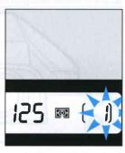
The frame counter indication in the viewfinder and on the LCD panel blink.
